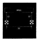
The first step in installing your OMNI unit is to position the poles. Begin with the end pole and be sure that it is plumb. Work from this pole as a reference point. (See diagram) When used away from the wall as a room divider or partitioning, be sure poles are in perfect alignment.
